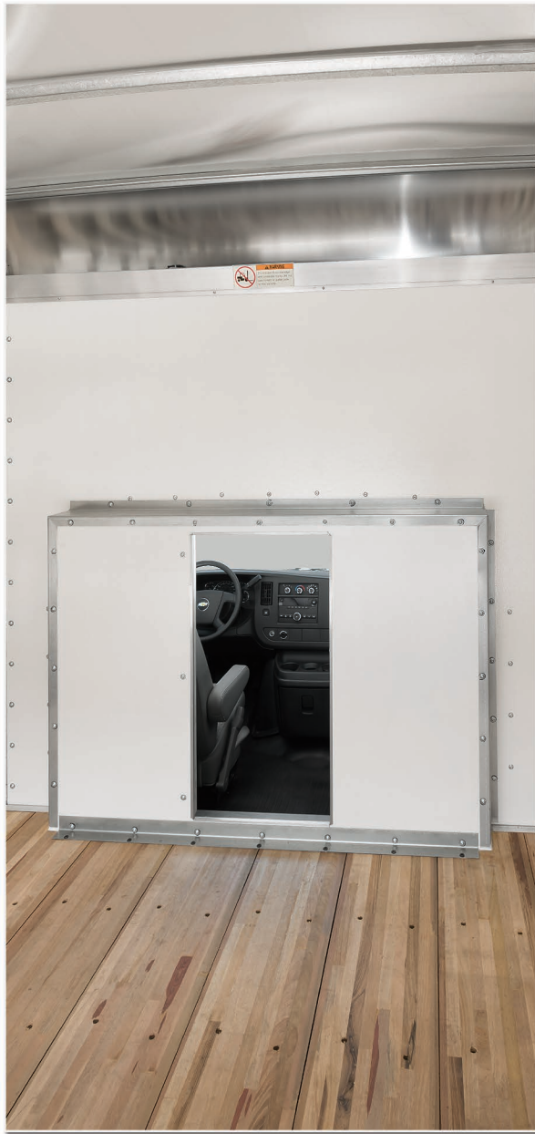
An option for a recessed bulkhead provides more room in the cab and easier positioning of the seat.
